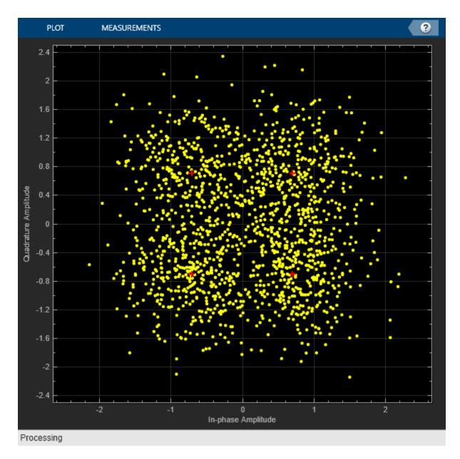
Demodulate the noisy symbols to obtain soft bits, convolutionally decode the soft bits, and display the number of erroneous bits.
