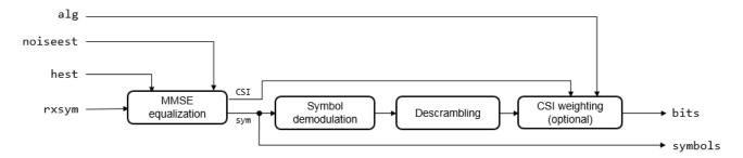
If the resource element grid across all possible EPDCCH antenna ports is input, the function extracts all EPDCCH resource elements and performs EPDCCH decoding for all possible EPDCCH candidate locations. The function assumes the input symbols were already equalized. Each EPDCCH candidate is descrambled individually during EPDCCH search.
