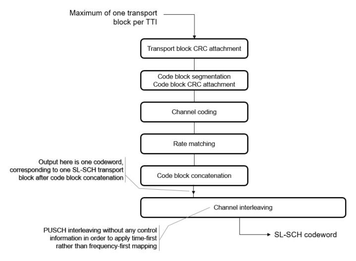
The SL-SCH transport channel codeword carrying the information bits of a single transport block is transmitted on the physical sidelink shared channel. Use the ltePSSCH and ltePSSCHIndices functions to generate the modulated symbols and populate the resource grid for transmission.
